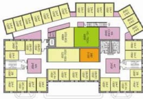
Rendering of proposed collaborative space (top) and diagram showing collaborative spaces (purple shaded areas) planned for the renovated Illini Hall. Images by De Stefano Partners.
